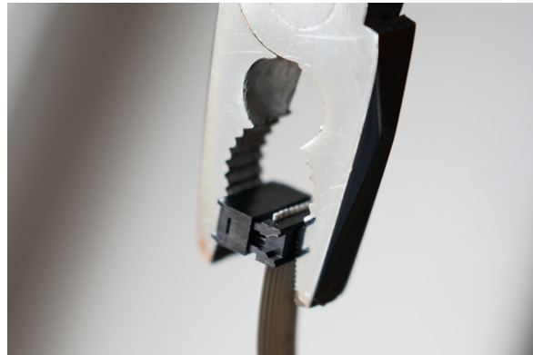
Figure 26: Fixation of the IDC connectors to the ribbon cable.
